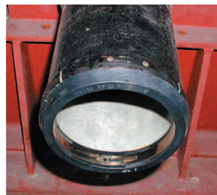
図14 試験後の防食ゴム Fig. 14 State of corrosion prevention rubber after an experiment (Polly-Pig passage test)
