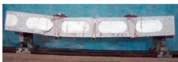
図13 ひび割れ発生状況(S1) Fig.13 Photo of crack initiation(S1)
