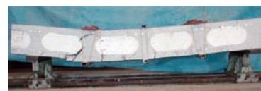
図14 ひび割れ発生状況(S2) Fig.14 Photo of crack initiation(S2)
