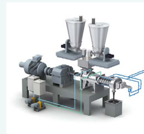
Continuous kneader (for the electrode slurry manufacturing process)
